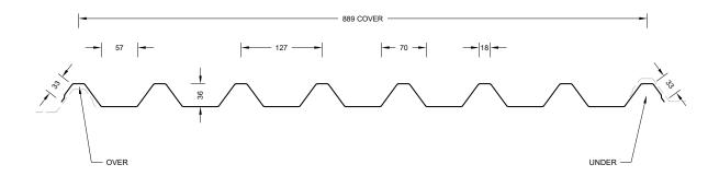
Designed for applications where protection from severe climatic conditions and maximum structural economy is required, the strong section properties of LT7® allow for wider purlin and girt spacings which add extra economy to building projects. It also has excellent water shedding characteristics as well as being perfect for low pitch roofs.
