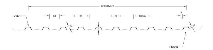
If versatility is what you are after, then Dimondclad<sup>®</sup> is the perfect cladding solution. Dimodclad's<sup>®</sup> clean efficient lines well concealed laps are excellent for both exterior and interior cladding. Dimondclad<sup>®</sup> Rib 20 features wide ribs with narrow pans for defined cladding lines.
