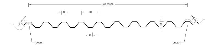
The clean-cut, striking appearance of V-Rib® makes it a very popular roofing and cladding profile used on a wide range of applications. The symmetrical sections have inherent strength characteristics which provide good tolerance to foot traffic as well as the title of the strongest drape curved roofing profile available. Where design criteria demand continuous length, economy and simple, speedy construction choose V-Rib®.
