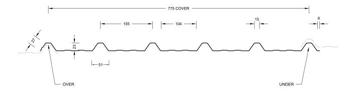
Dimond Six Rib® offers clean lines and a strong visual appeal. Six Rib® is already suited for cladding applications down to 4 degrees. Distinguishes itself with its lower rib height giving it a lighter weight looking appearance.
