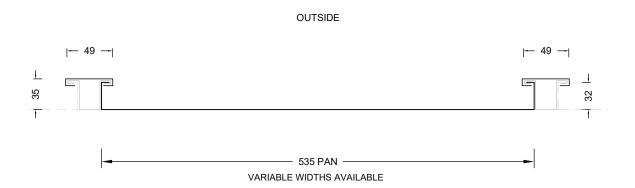
With shadowed elegance, this simple but stylish profile can be formed from steel-based materials as well as copper and zinc. Creating a slightly softer finish and larger effect than Eurotray® Roll Cap, Eurotray® Roll Seam can be machine curved to allow for more expensive detailing.
