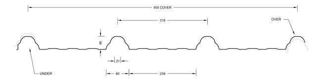
DP955° is designed not only to be stronger than traditional profiles but also more cost effective and faster to install. Its design provides stronger ribs to protect against buckling and wide style pan to allow for safe foot placement. With a wider cover width of 955mm, fewer DP955° sheets are required to be installed, saving both time and money. DP955° soriginal look creates a distinctive and diverse design unlike traditional profiles ensuring a unique finish.
