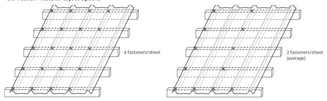
Can be installed over plastic cavibat battens.
