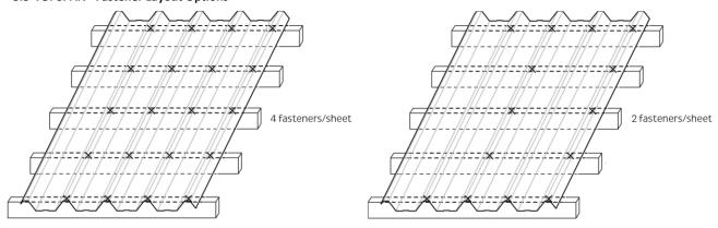
Can be installed over plastic cavibat battens.
