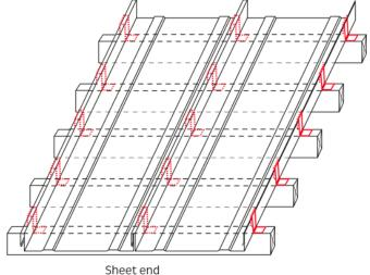
Can be installed over plastic cavibat battens.
