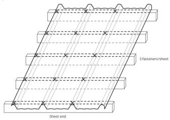
Can be installed over plastic cavibat battens.
