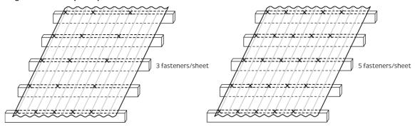
Can be directly installed over plastic cavibat battens.
